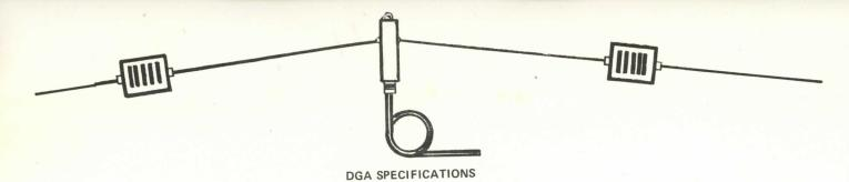
The DGA Antennas when cut to the center of each band measure from a minimum of 50 ft. to a maximum length of 106 ft. (plus 6 ft. minimum of rope on each end) the traps are high Q and use no. 12 and no. 14 gauge wire. The standard coaxial cable supplied is RG-59/U at 72 ohms. (Except for the DGA - 152040 which is supplied with RG-8/U at 52 ohms)
